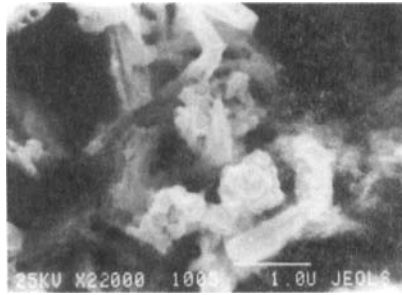
FIGURE 10 SEM photograph of sample of 0.5- \mu\text{m} tungsten powder. The magnification is 22000x.
